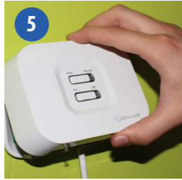
5 Clip the front of the unit back on by aligning the fittings and pushing into place.
